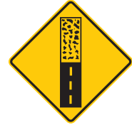
Pavement ends ahead
