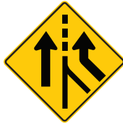
Road merges with another road — added lane to the right ahead
