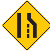
Right lane ends ahead
